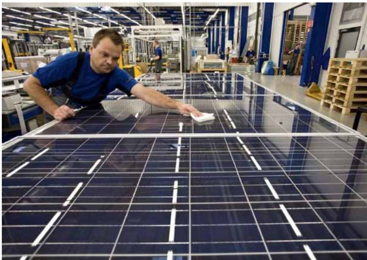
Cleaning of finished solar modules
